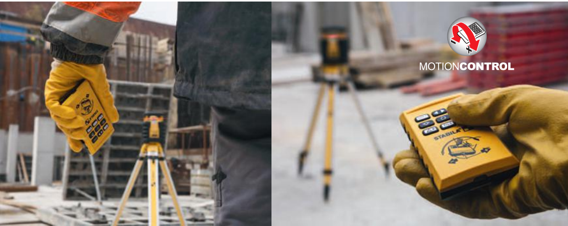
The RC-LAR350 remote control with MOTION CONTROL: intuitive control of all laser functions in no time at all
