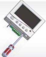
Carefully separate the front half of the thermostat from the back plate by placing a small flat head terminal driver into the slots on the bottom face of the thermostat.
