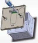
Screw the thermostat back plate on to the back box
