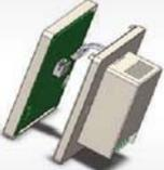
Carefully unplug the ribbon connector which is plugged in to the front half of the thermostat
